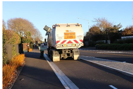
Figure 6: Kerbside waste collection vehicle straddling a cycle lane to collect waste
